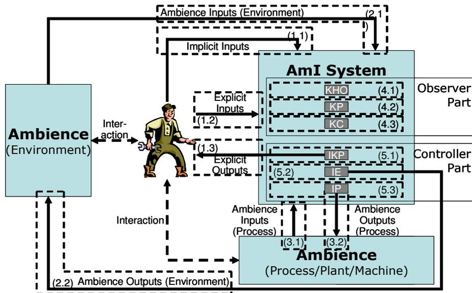
Figure 1: Reference model for AmI in manufacturing industry.
