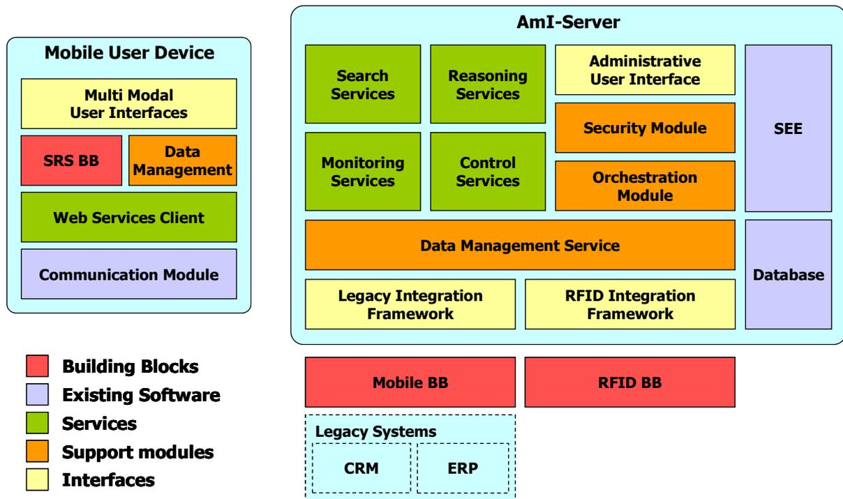
Figure 2: AmI Software Architecture.
